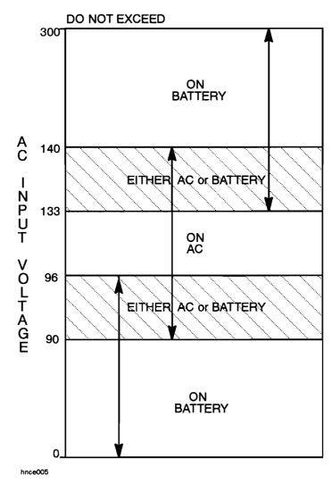
Figure 2-6. 100 to 120 Voltage Range (50/60 Hz)
