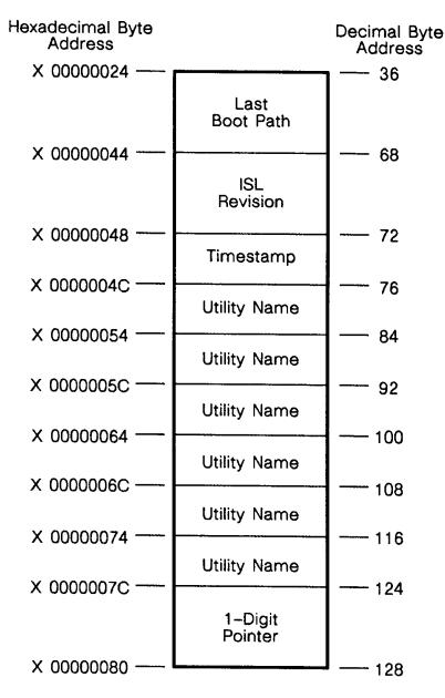
To read an NVM location, enter the ISL READNVM command and enter the hexadecimal or decimal address. The output is always in hexadecimal. In the following examples, addresses are referred to in decimal notation and the output is in hexadecimal notation.
