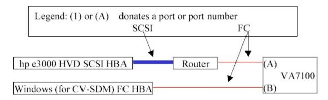
Notes: Recommend that HP e3000 be connected to the "performance port" of the VA7100, generally this is the port on Controller 1 of 2.
