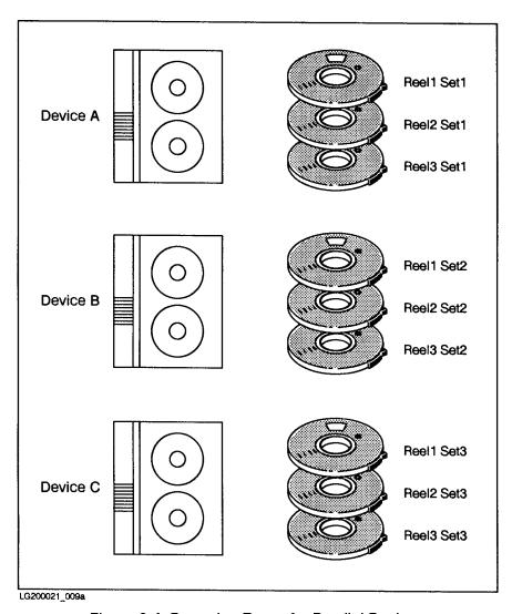
Figure 3-4. Preparing Tapes for Parallel Devices
