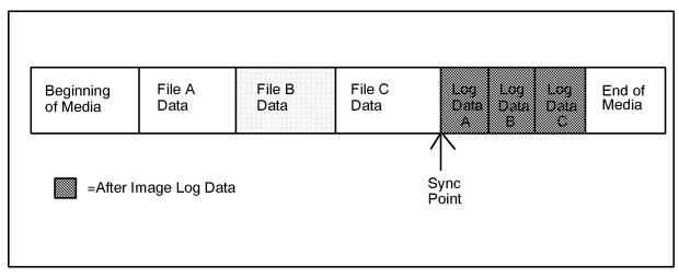
Figure 7-2. Backup Created with Sync Point at the End
