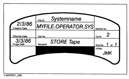
Figure 3-2. A Correctly Labeled Tape
