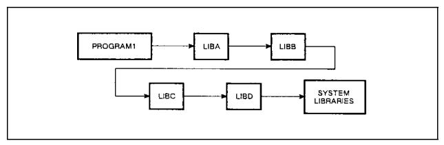
Figure 3-1. Illustration of a Load Time Binding Sequence.
