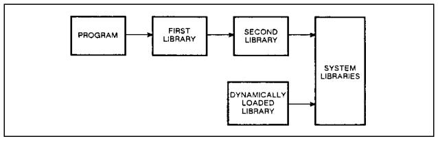
Figure 3-2. Illustration of Run Time Binding of an XL.
