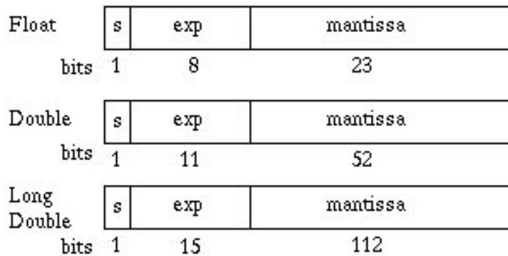
Figure 10-1 Internal Representation of Floating-Point Numbers
