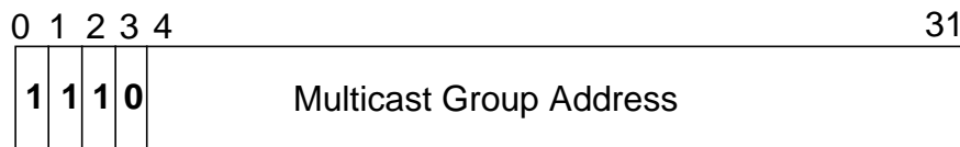
Figure 9-2 Class D IP multicast address format
