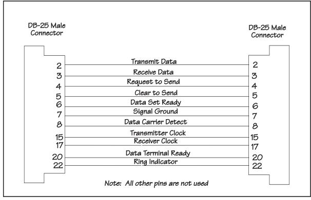
Modems and modem eliminators provide transmit clocking signals on EIA-232 (RS-232) pin 15 and receive clocking signals on pin 17.
