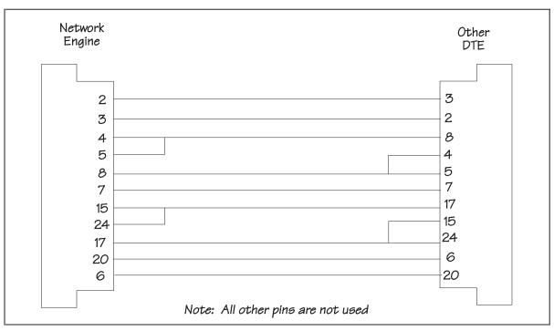
If the other DTE equipment provides a clock signal on EIA RS-232 pin 24 (External Transmitter Clock), the cable between the DTE equipment and the Network Engine's Modem port should be wired as shown in the diagram below:
