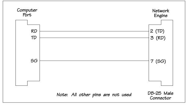
The Network Engine is an RS-232 DTE device - any cable that may be used to connect a terminal to your HP 3000 may be used to connect the Network Engine as well. A cable containing all 25 pins wired straight-through (no crossovers) may be used.
