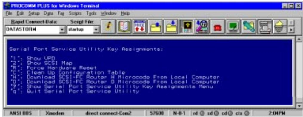
Figure 4-4. Serial Port Menu for Host Router
