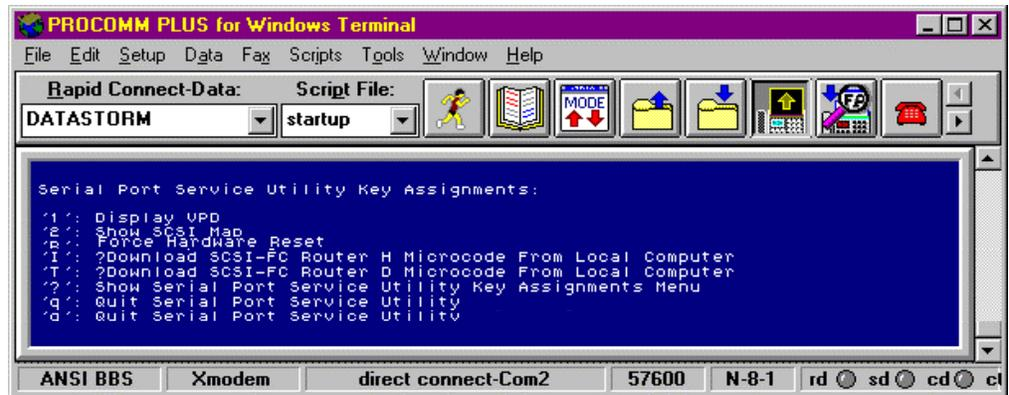
Figure 4-5. Serial Port Menu for Device Router
