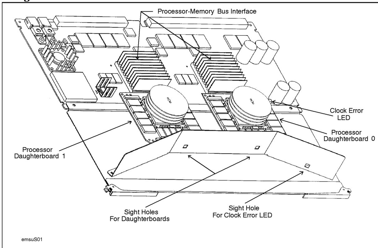
5. Remove the processor card with only one processor daughterboard:
