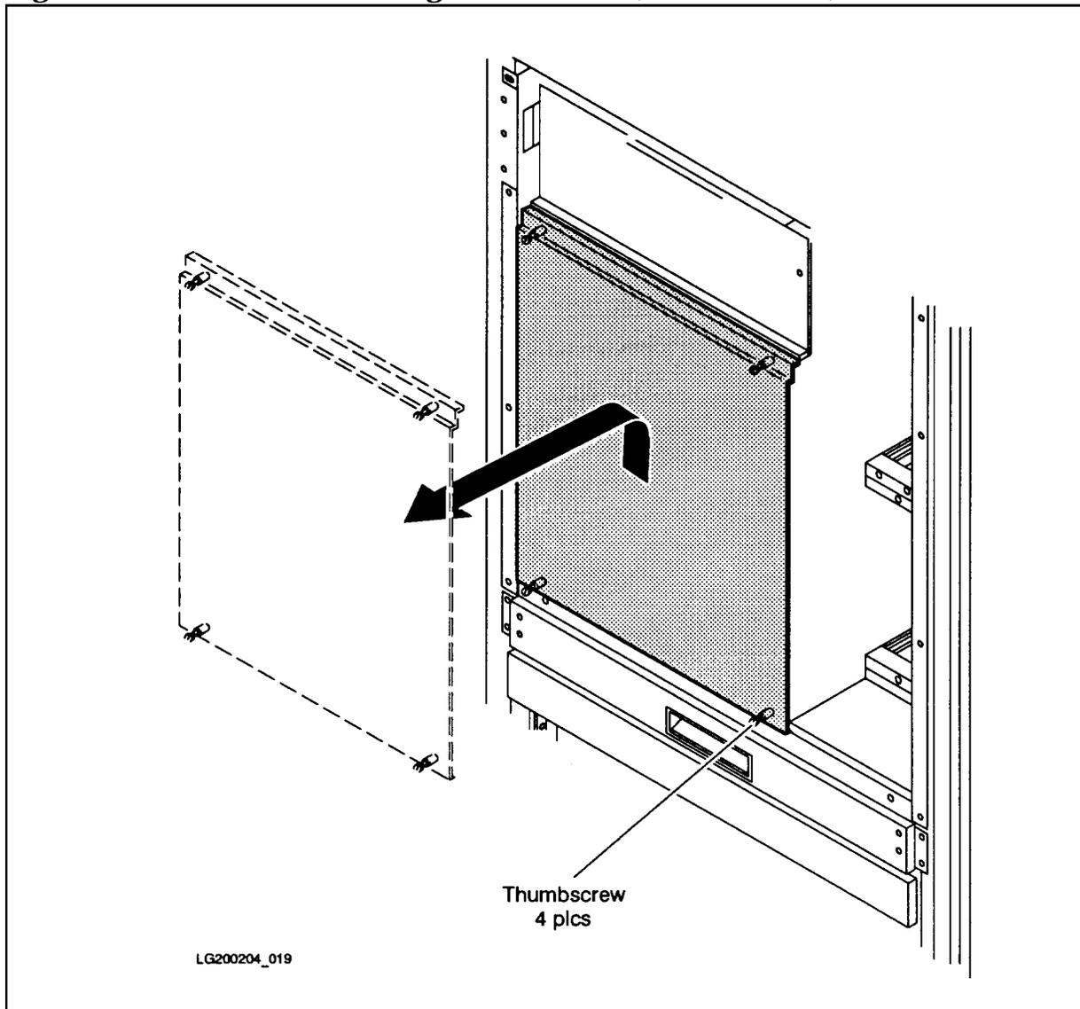
**To remove the cover plate from the front PMB card cage:**
