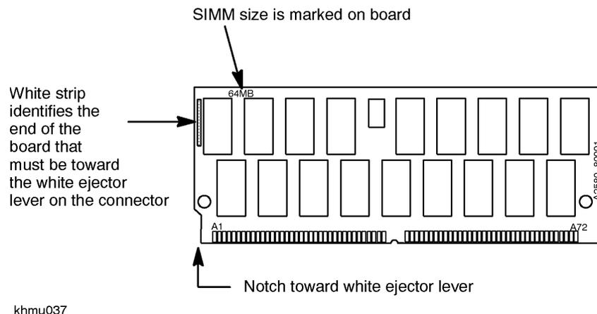
A module is a pair of SIMMs or DIMMs. Memory for your system is purchased and installed only in modules; never install just one SIMM.
