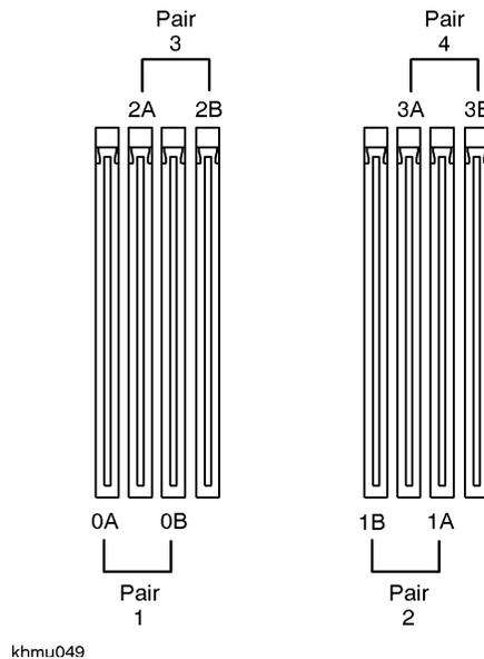
The largest-sized modules (SIMM pairs) are installed in the lower number slots, followed by smaller-sized modules.
