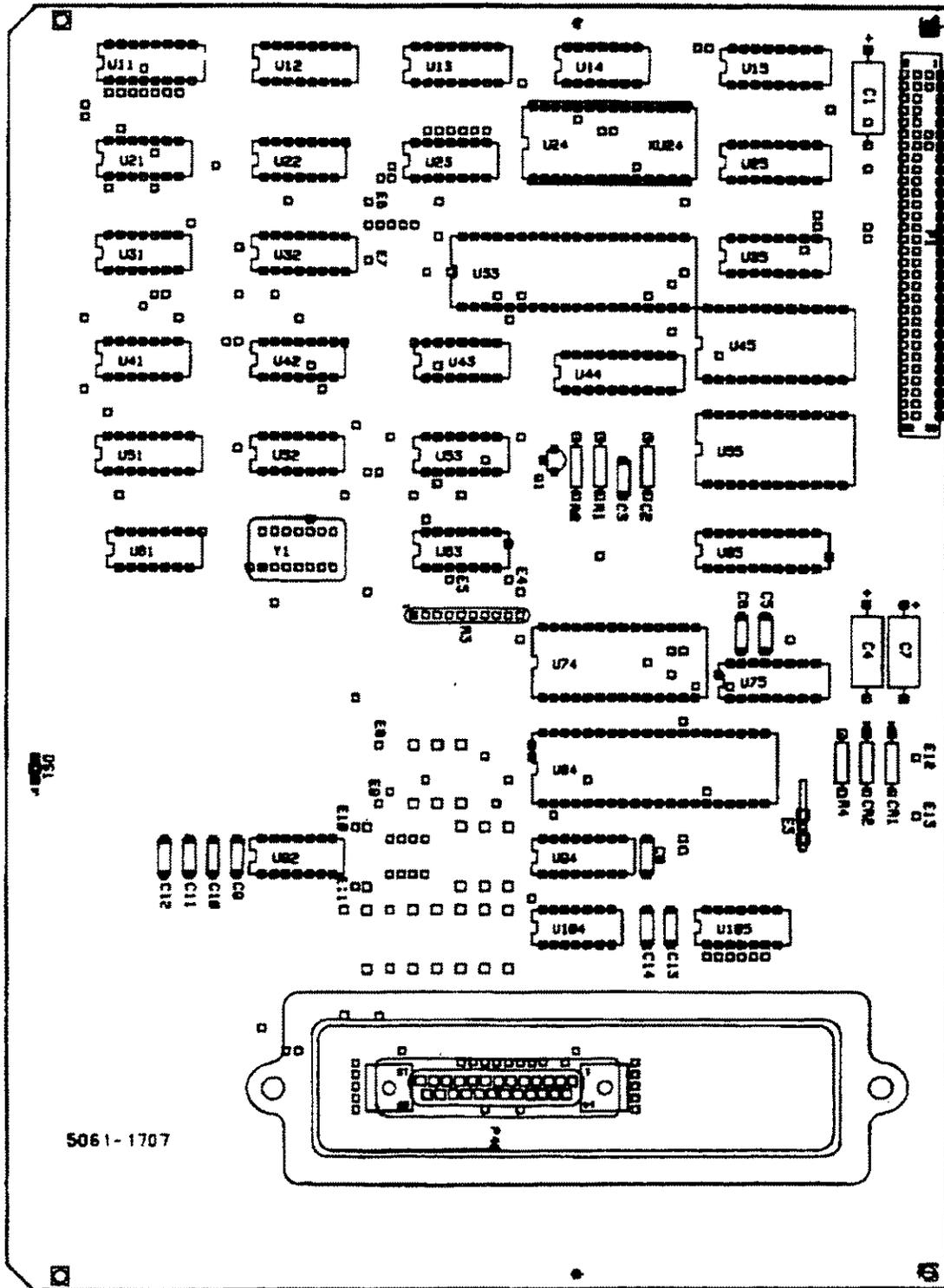
Figure 4-2. Serial Interface PCA (5061-1707), Parts Location
