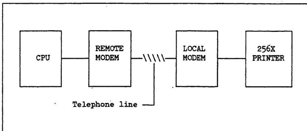
Figure 4-1. Modem Loopback Test 32
