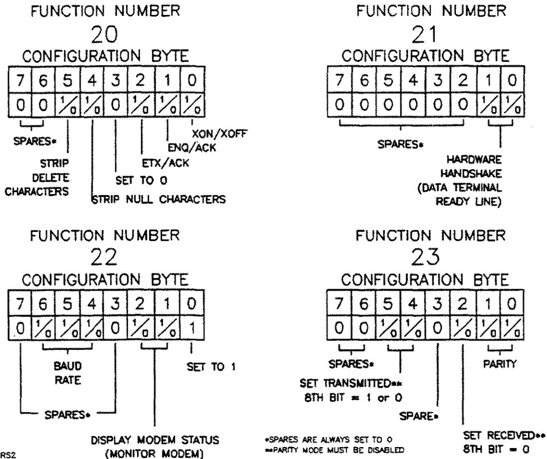
Figure 2-3. Configuration Bytes
