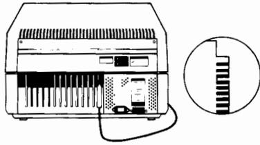
**Step 2.** Raise the unit's hinged rear access cover (two rotating latches hold it in place) and connect the keyboard cable hood connector to the printed circuit card. The printed circuit card has been notched to match the cable connector.
