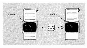
You can clear the portion of a line to the right of the cursor by holding the var. key down and pressing CLEAN OBSPLY.
