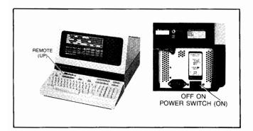
STEP 3. (Optional) You should also press the  $\frac{1}{1657}$  key. If the terminal beeps and displays a test pattern similar to that shown on page 8-2, the terminal is working properly and is ready to use.
