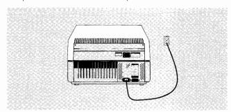
STEP 5. MAKE SURE THAT YOUR VOLTAGE MATCHES THE TERMINAL'S REQUIREMENTS (either 115V or 230V, see the rear panel label). Plug the 3-prong power connector into your power outlet.
