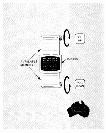
The west and whose keys allow you to move the display 24 lines (a whole screen) forward or backward in memory. When you press these keys the information presently displayed is replaced with the next (or previous) 24 lines of memory.
