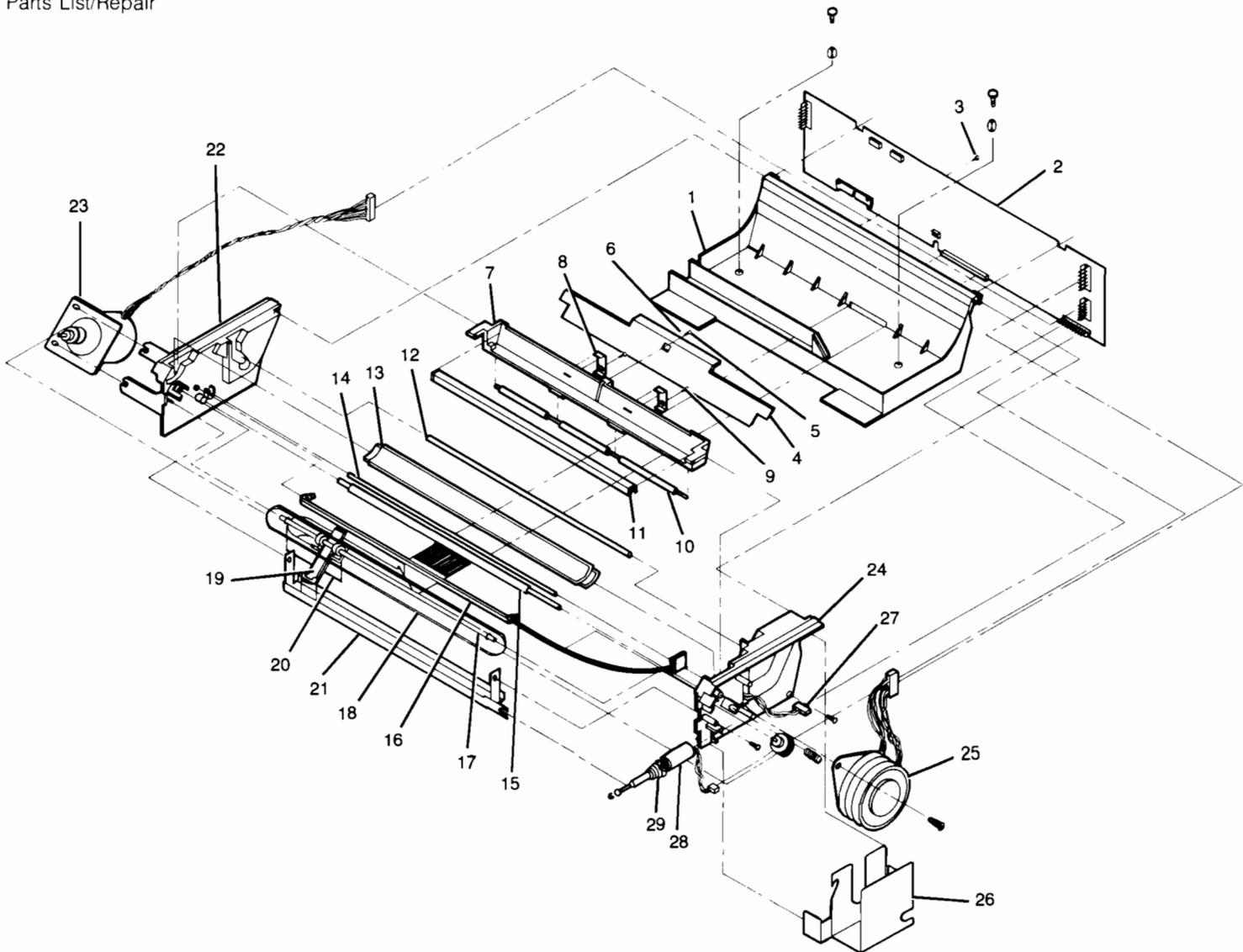
Figure 7-17. TPM, Exploded View
