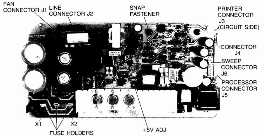
Figure 2-6. Optional 120 Watt Power Supply PCA
