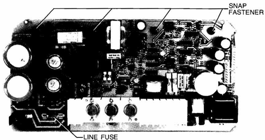
Figure 7-9. Power Supply PCA (Terminals with Printers)
