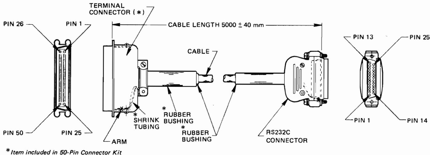
Figure 2-17. 13222 Series Cable Fabrication (Port 1)
