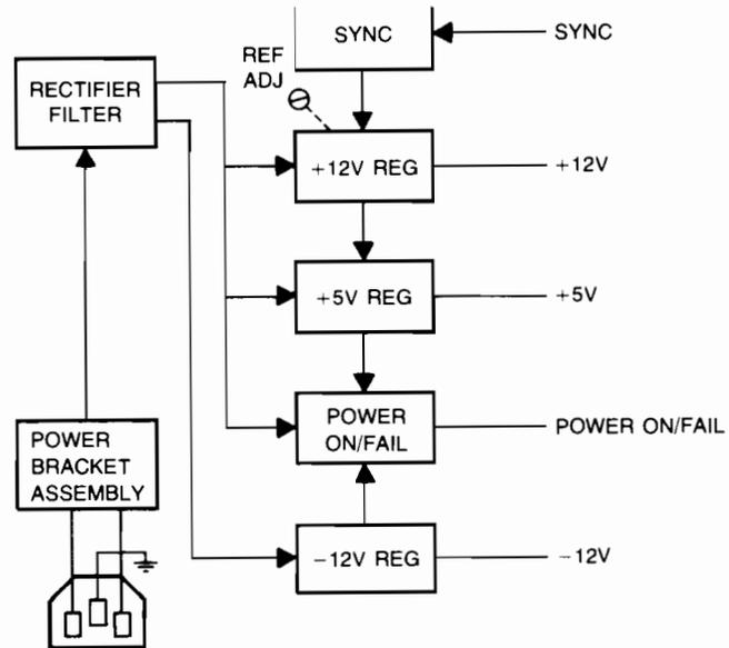
Figure 8-5. 65 Watt Power Supply, Simplified Block Diagram
