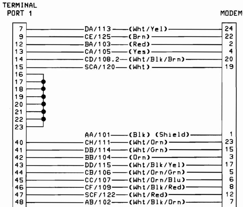
Figure 2-8. 13222M (European Modem) Cable Wiring
