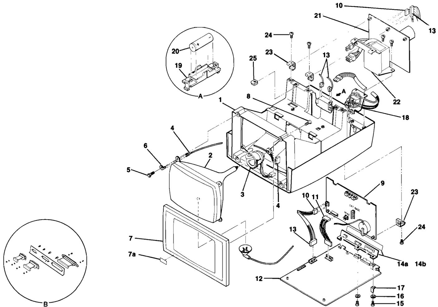
Figure 7-16A. Mainframe, Exploded View (Standard)
