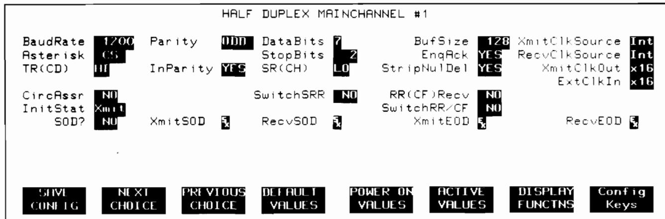
Figure 3-6. Half Duplex Main Channel Configuration Menu
