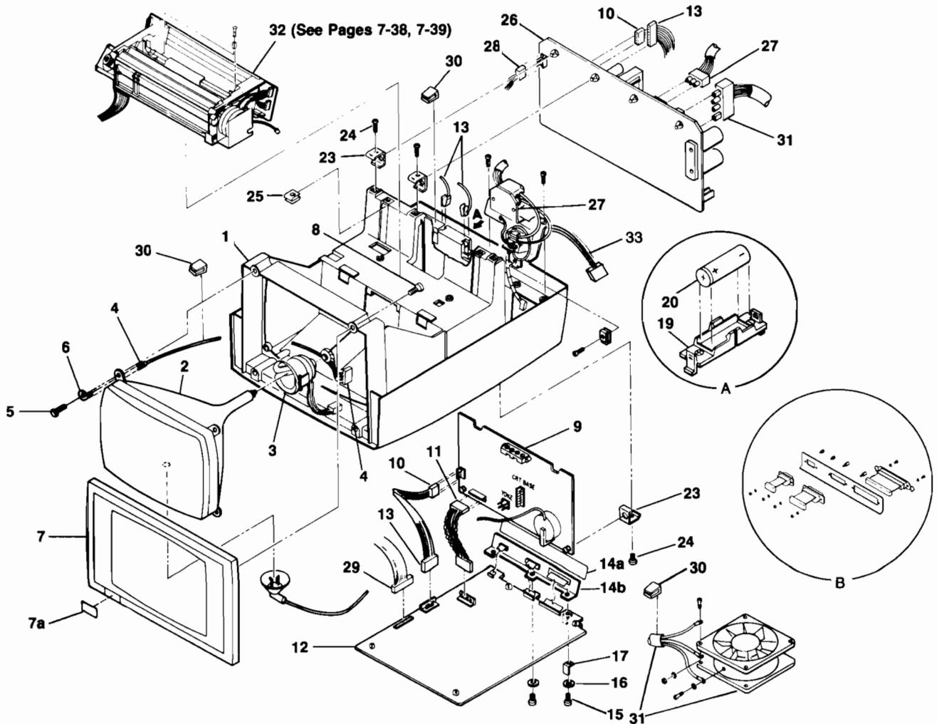
Figure 7-16B. Mainframe, Exploded View (Option 50)
