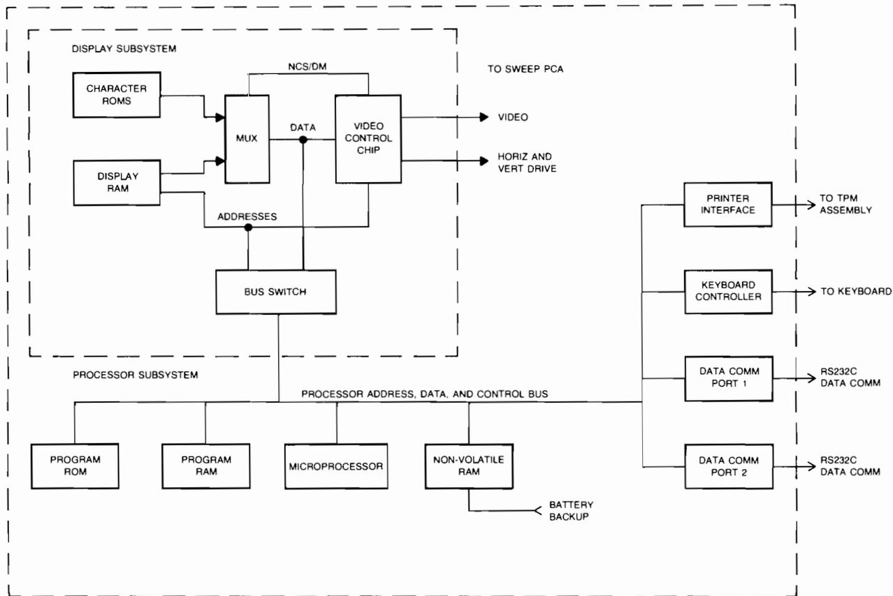
Figure 8-3. Processor PCA Block Diagram
