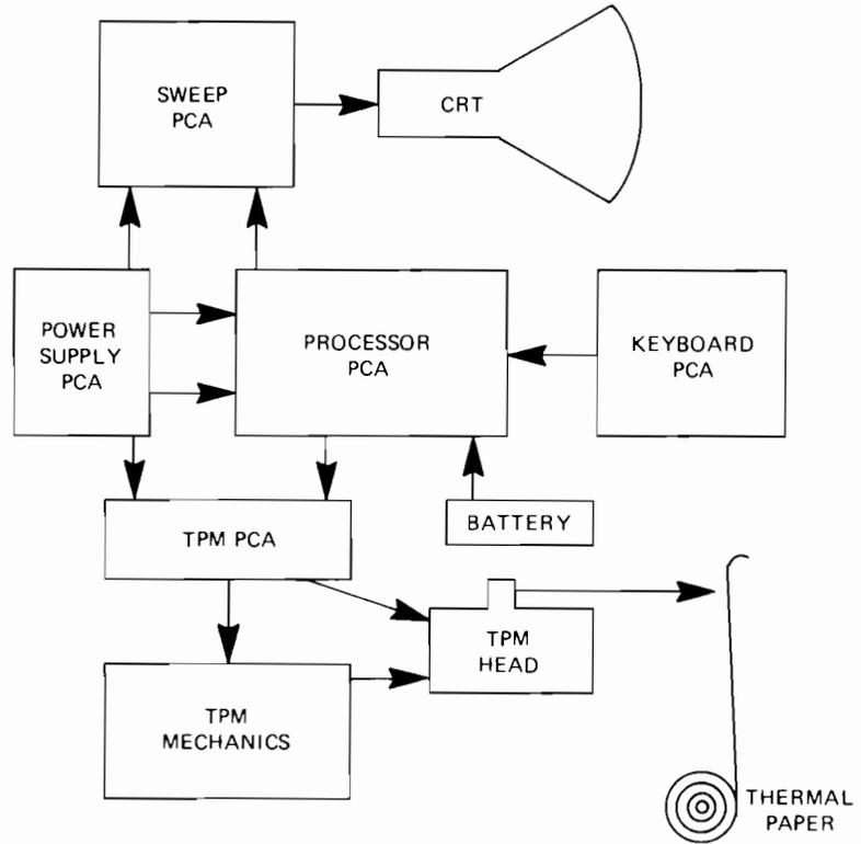
Figure 8-2. Simplified Block Diagram for Terminals with a Printer
