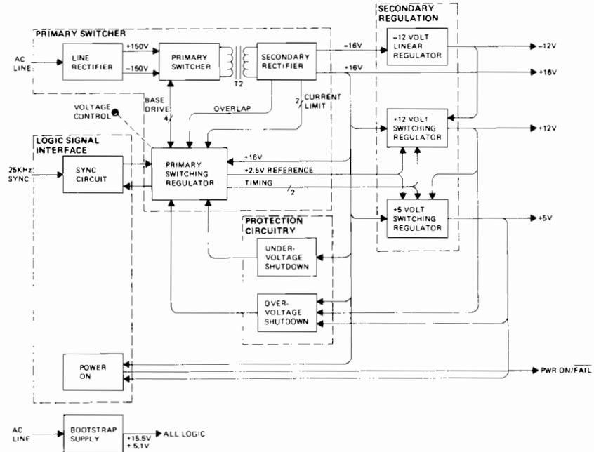
Figure 8-6. 120 Watt Power Supply, Simplified Block Diagram
