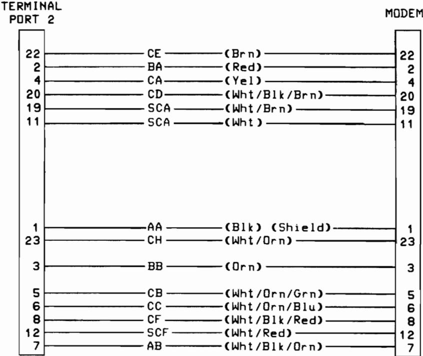
Figure 2-15. 13242N (U.S. Modem) Cable Wiring
