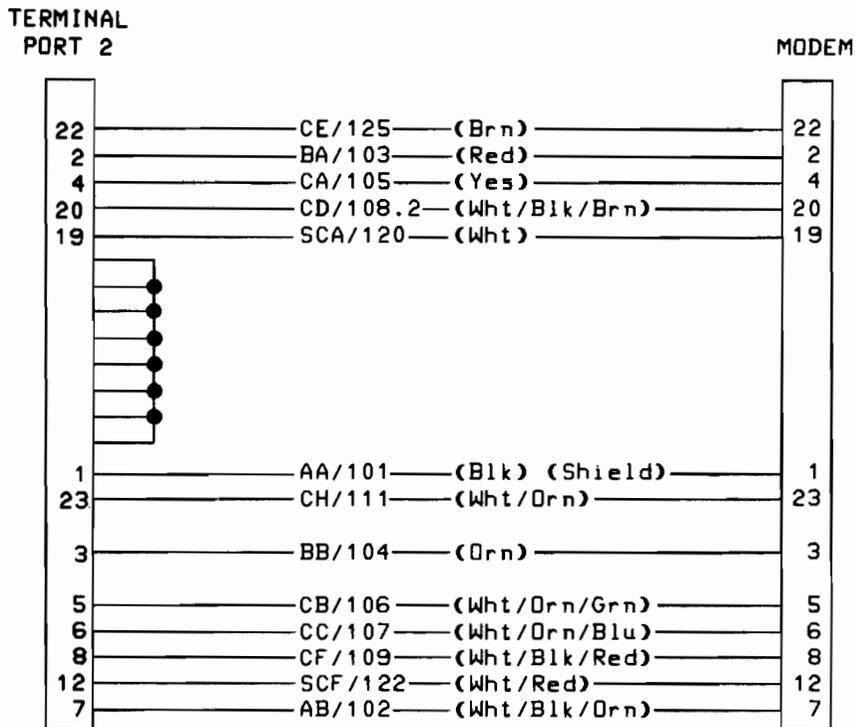
Figure 2-14. 13242M (European Modem) Cable Wiring
