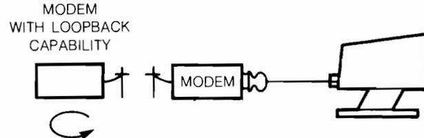
**REMOTE MODEM TEST SETUP**
