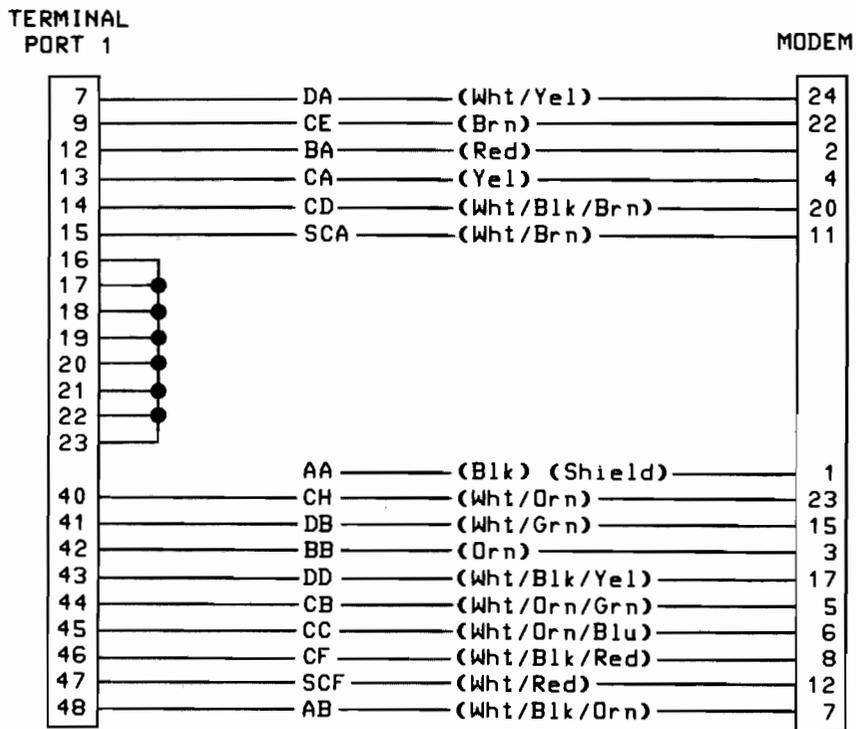
Figure 2-9. 13222N (U.S. Modem) Cable Wiring
