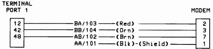
Figure 2-11. 13222Y (Three Wire/Male) Cable Wiring
