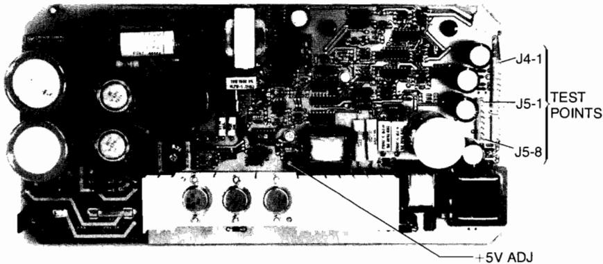
Figure 5-2. Test Points for Terminals with the Printer Option and +5V Adjustment Locations
