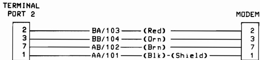
Figure 2-16. 13242Y (Three Wire/Male) Cable Wiring
