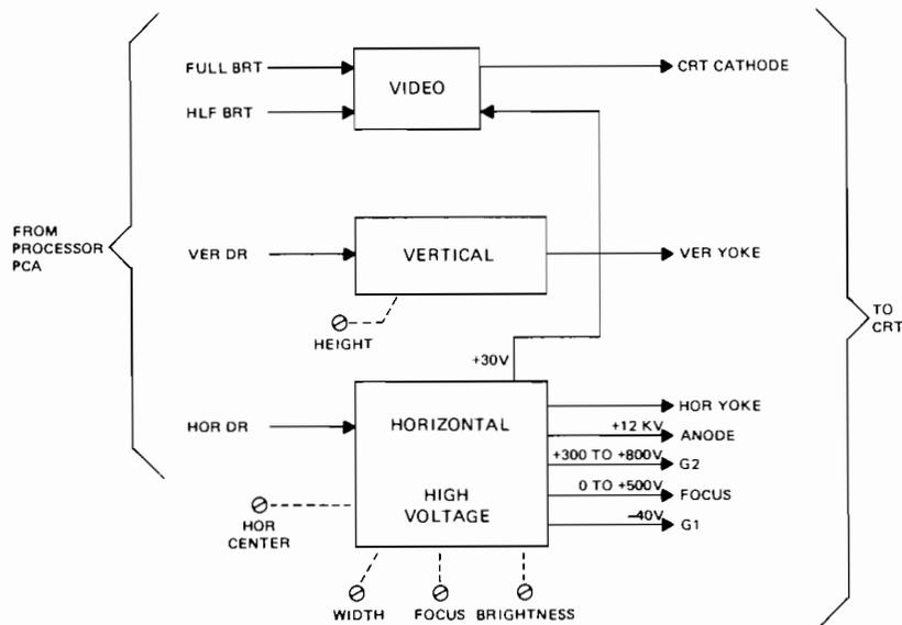
Figure 8-4. Sweep PCA, Simplified Block Diagram
