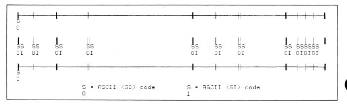
Figure 5-5. Use of Shift-In and Shift-Out Codes
