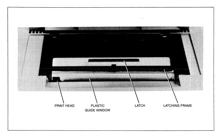
Figure 10-3. Printer Mechanism
