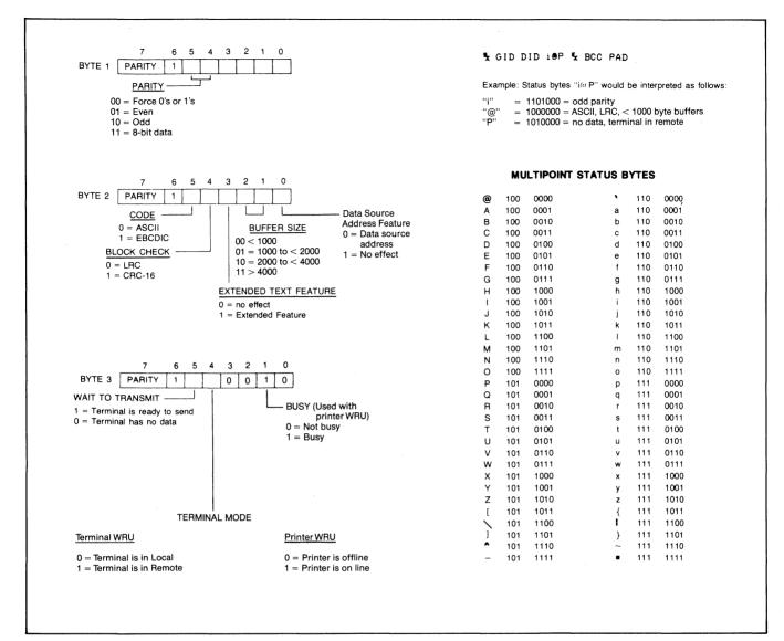
Figure 7-24. Configuration Status Byte Contents
