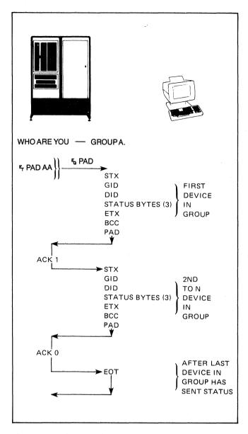
Figure 7-23. Typical Configuration Status Request and Response Sequence
