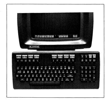
Figure 1-3. Function Keys and Screen Labels
