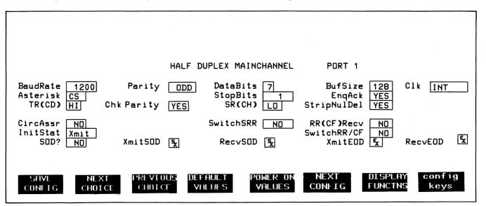
Figure 7-10. Half Duplex Main Channel Configuration Menu
