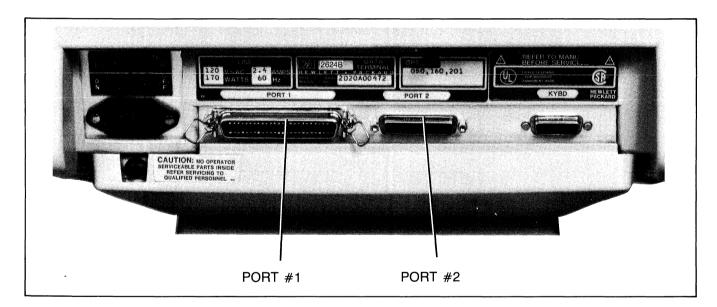
Figure 7-4. HP 2624B Display Terminal, Rear View
