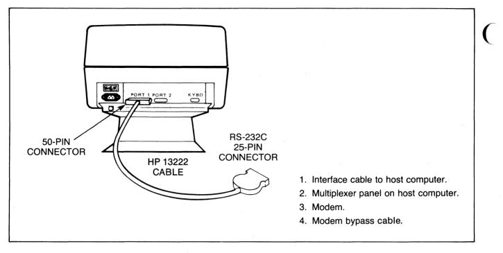
Figure 7-5. Port #1 Cabling (HP 13222 Cables)
