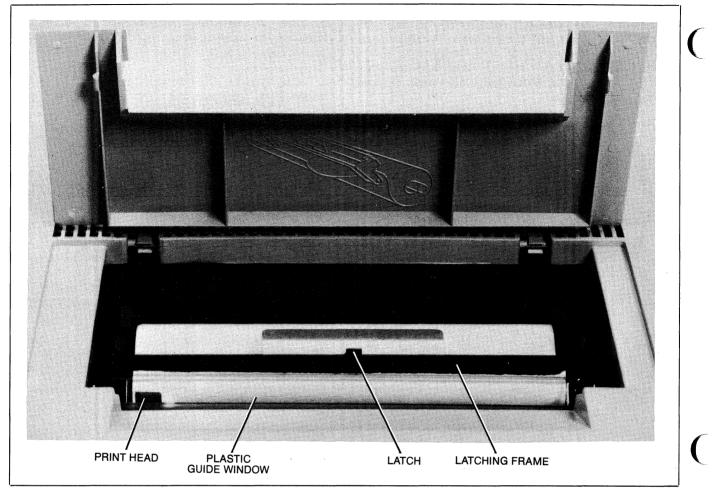
Figure 6-4. Integral Printer Mechanism
