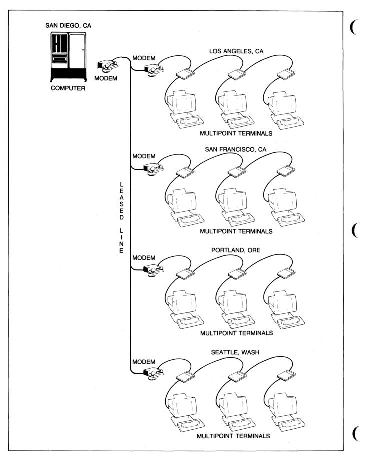
Figure 7-3. HP Multipoint Configuration (Leased Line, Multidrop)
