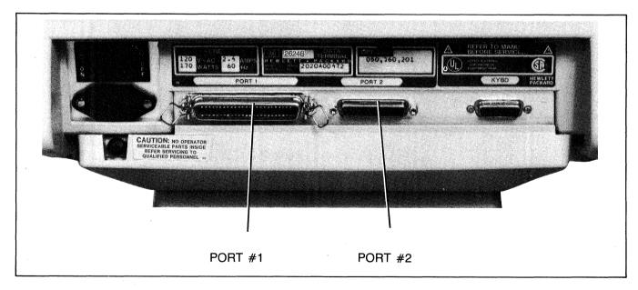
Figure 7-12. HP 2624B Display Terminal, Rear View
