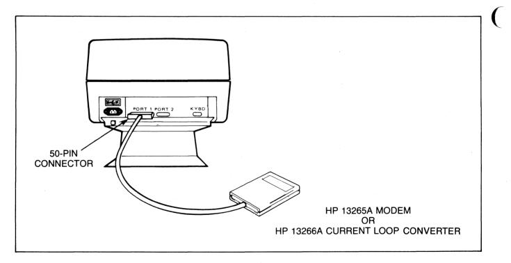
Figure 7-6. Port #1 Cabling (HP 13265A Modem or HP 13266A Current Loop Converter)
