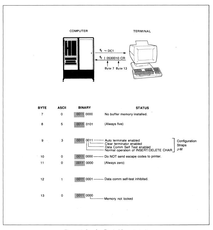
Figure 8-2. Secondary Terminal Status Example
