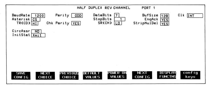
Figure 7-11. Half Duplex Reverse Channel Configuration Menu
