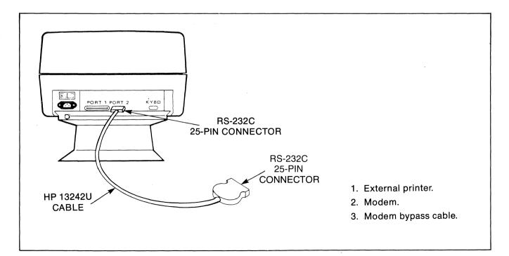
Figure 7-14. Port #2 Cabling (HP 13242 Cables)
