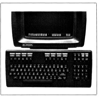
Figure 3-1. Screen-Labeled Function Keys
