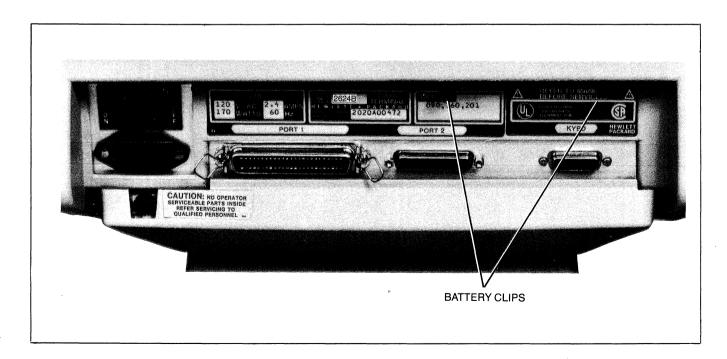
Figure 10-1. Battery Location, Rear Panel
