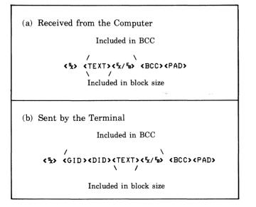
Figure 7-25. Examples of Block Transmissions
