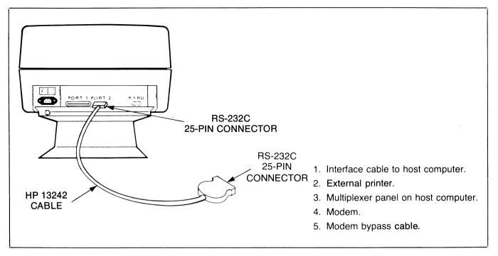
Figure 7-5. Port #2 Cabling (HP 13242 Cables)
