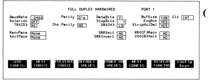
Figure 7-8. Full Duplex Hardwired Configuration Menu
