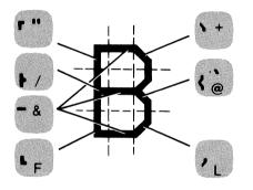
As with any of the alternate character sets, you enable the Large Character set with a **<SD>** control code (control-N) and disable it with a **<SI>** control code (control-O).
