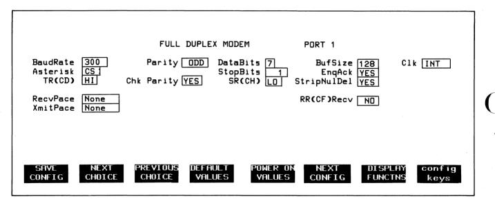
Figure 7-9. Full Duplex Modem Configuration Menu
