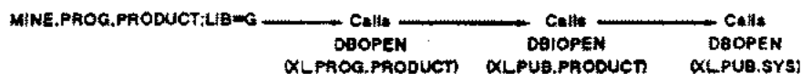
Figure 3 - 4: The flow of control when libraries are copied to the program account
