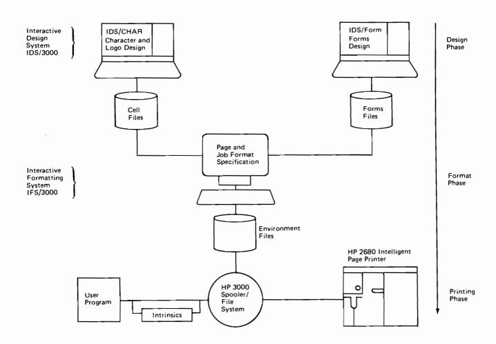
Figure 1. HP2680 Laser Printing System
