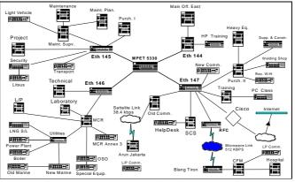
Figure 3. Arun Network Hub Segmentation
