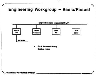
Many engineering applications require use of computers to control various types of test and measurement equipment. HP offers several computers optimized for this task. One widely used computer is an HP 9000 Series 200 or 300 running the BASIC operating system (Rocky Mountain BASIC). The HP network for these systems is the Shared Resource Manager (SRM). The SRM features peripheral and file sharing and allows operation of the workstations without local discs.
