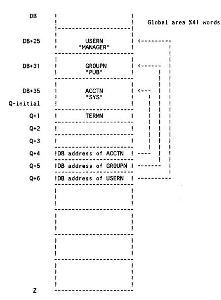
Next we must find where the values of Q+4, Q+5 and Q+6 are set and patch the code to load the new DB+ values we have allocated instead of the ones generated by the compiler.
