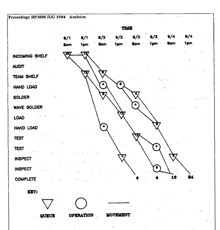
Figure 7. "Spencer Diagram". In this example the boards from this work order were first observed in the incoming queue at 9 a.m. on 9/1. By 1 p.m. on 9/4 all boards had been completed. The total boards observed at each time are equal to 24. Data collected in this manner over many work orders can be summarized to yield an accurate picture of how material flows through the process.
