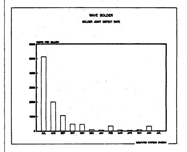
Figure 2. Wave Solder Defect Rate. This shows the dramatic decline of solder defects over a 13-month period. The large increase in June, 1983, was attributed to one lot of boards which had sat unattended on a shelf for several weeks.
