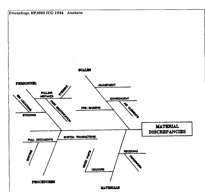
Figure 5. Cause and Effect Diagram Showing Possible Causes of Material Discrepancies. Brainstorming is a good technique for identifying possible causes for a problem such as this.
