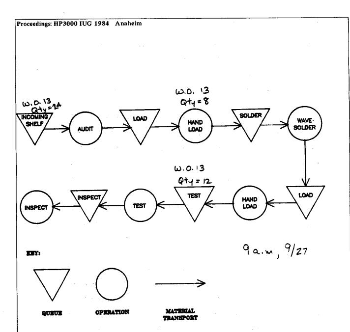
Figure 6. Process Flow Diagram. This example shows the process flow diagram used for data collection. The work order number and quantity of boards found in each step of the process has been recorded. In the example 24 boards from work order number 13 are held in the incoming queue.
