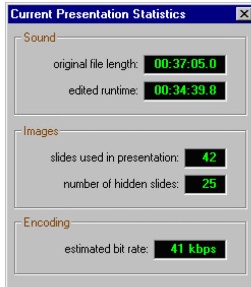
Fig 4.8. The current statistics form, listing the original file length, the currently edited runtime, the number of slides used in the presentation, the number of slides that have been hidden, and the estimated encoding bit rate that will result from these editing decisions.
