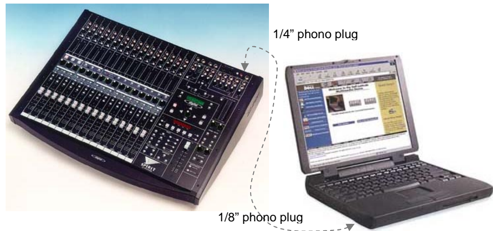
Fig. 2.2. A standard professional-quality stage audio mixer board and the necessary connecting cable to your laptop.
